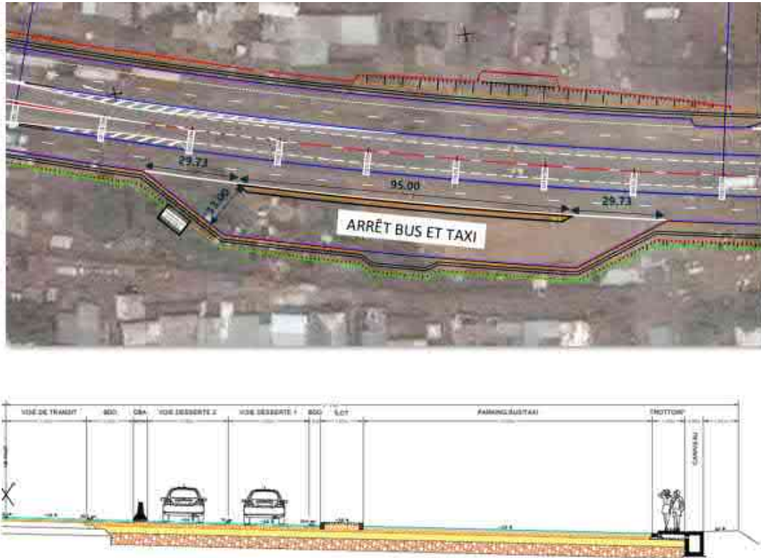
FIGURE 2-14: EXAMPLE OF BUS STOP CONFIGURATION
